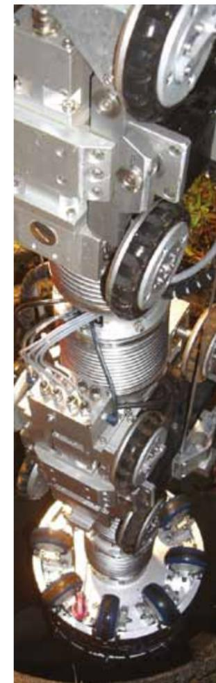
The SLOFEC method is based on the eddy current principle in combination with a magnetic field. From the inside of the pipe any possibly concealed corrosion on the outside of the pipe is detected. The detection capacity of this technology utilises its advantages in thick-walled, cast iron or even coated pipes.
